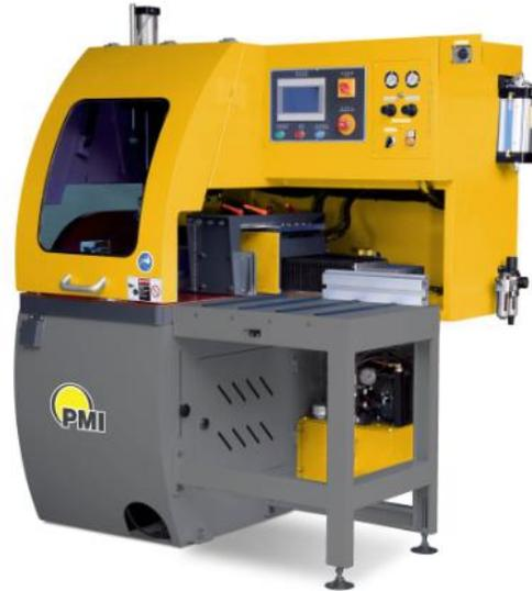
The PMI-18 DB-Type Automatic High Production Cutoff Saw is designed for sawing Aluminum Extrusion and Other non-ferrous metals. The saw's powerful 7.5 HP saw motor allows it to cut quickly and accurately. The gripper vise is ball screw with servo motor driven so the saw's indexing system is designed for accurate cut lengths. The 5.7" touch screen control allows for easy job setup.
