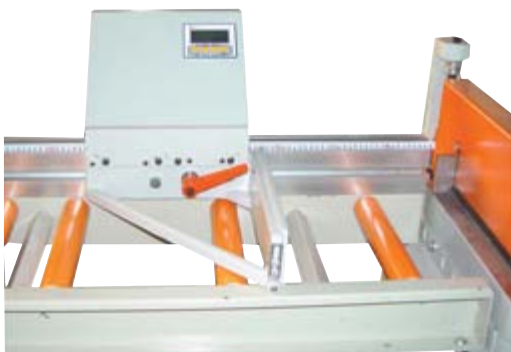
OUTFEED ROLLER TABLE (MAGNETIC SCALE WITH LCD DISPLAY)
