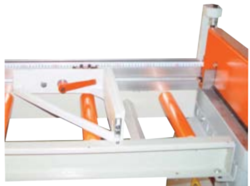
OUTFEED ROLLER TABLE (COMMON SCALE WITH STOP)
